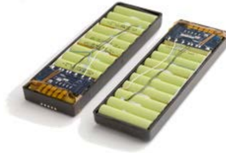
Figure 3: Lithium Ion Battery Cells Inside Enclosure
